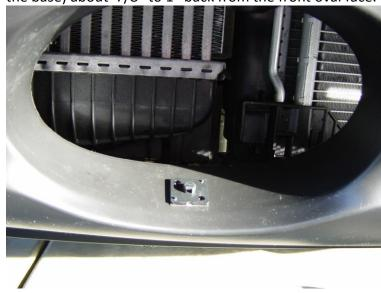
Attach oval grill assemblies to intakes using the Tie Wraps. You'll want to position the grills in place and carefully pull on Ties until both top and bottom are secured snug. See video here: <a href="http://www.youtube.com/watch?v=dls\_a5O6KkE">http://www.youtube.com/watch?v=dls\_a5O6KkE</a> which shows how the ties are fed through the grill to secure to the air intake ports.
