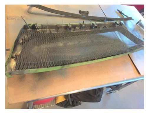
Most of the lower edge can be folded down and sandwiched under the metal grill bracket once it's reinstalled. So the best way to do this is to cut a straight line in from the mesh's edge to the grill's lower corner. This makes the bottom of the mesh into a flap you can fold down over the bottom edge.
