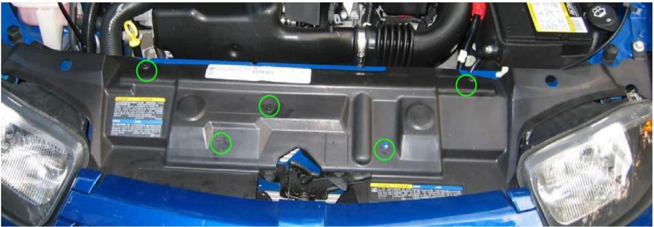
4. The push screws are located in the circled areas or possible elsewhere depending on model.
