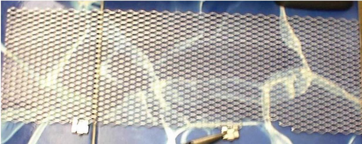
4. Now turn the grill around and tighten down the clamping part of the clip to the desired tension. Just take your pliers and close the gap down as far as you want. If you don't tighten them down enough, they will not hold and if you tighten them too much it will be hard to install.
