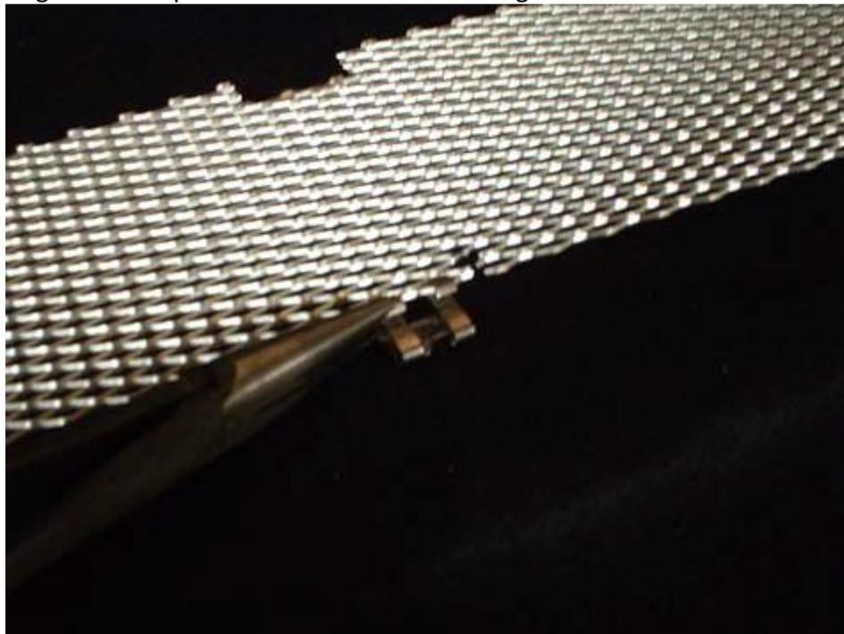
d. Then tighten down the back part of the clip. If you do not tighten down enough, the clip will not hold well on the bumper. If you tighten down too much, it may be difficult to install.
