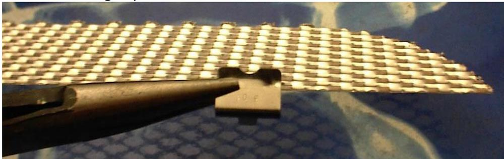
d. The tighter you clamp on the back the better the hold will be, but do not clamp down too hard or it will be difficult to install.
