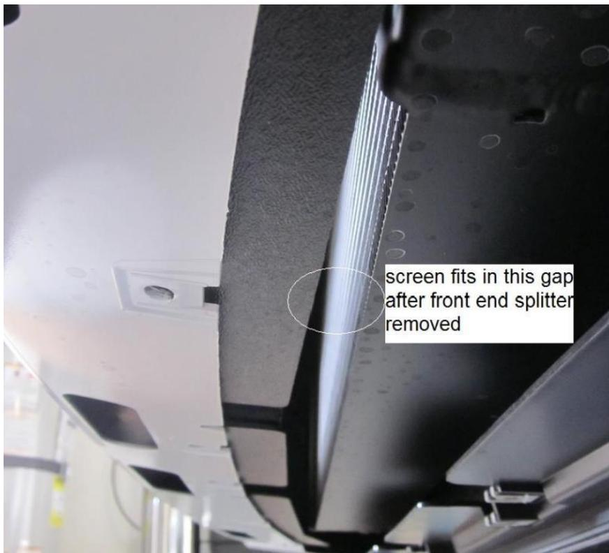
Insert mesh from below, insuring proper side to side fitment. If too tight, trim one row of hexes off with snips and reapply rubber gasket. The top of the mesh fits nicely into the gap under the white fender cover and the black styrofoam bumper filler.
