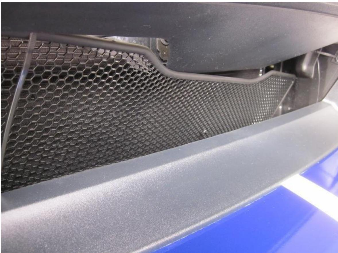
Place 3 self adhesive retention tabs on the 3 plastic tabs on inside of lower opening, 2 on top by shoulders and 1 on each side. Attach zip ties on the tabs, leaving ends open.
