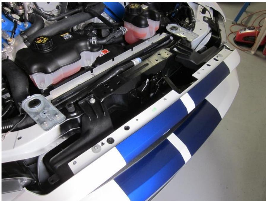
You can see into the space behind grille opening, but cannot put mesh in from above due to an attached tab from air deflector to latch; you must work the mesh into place from the opening in the grille front.
