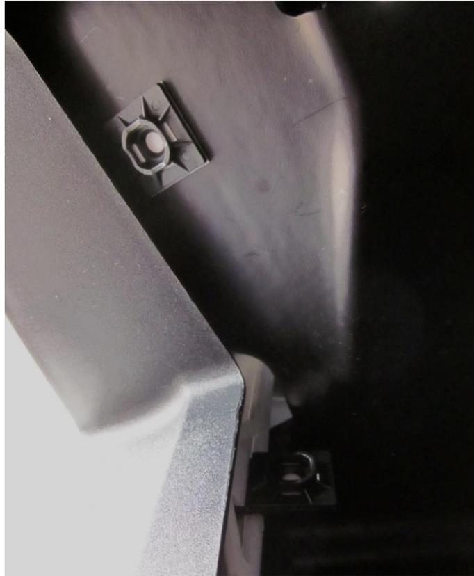
When mesh is in place, close zip ties and trim tail. Replace hood splash guard and the top portion of the mesh install is complete.
