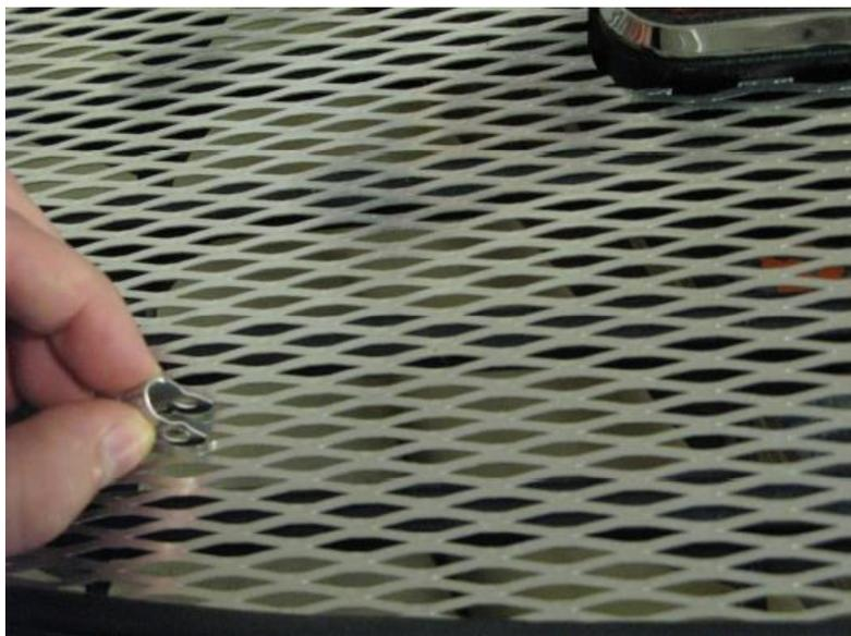
4. Run a cable tie through the holes in the clip. The tie should straddle on of the horizontal bars.
