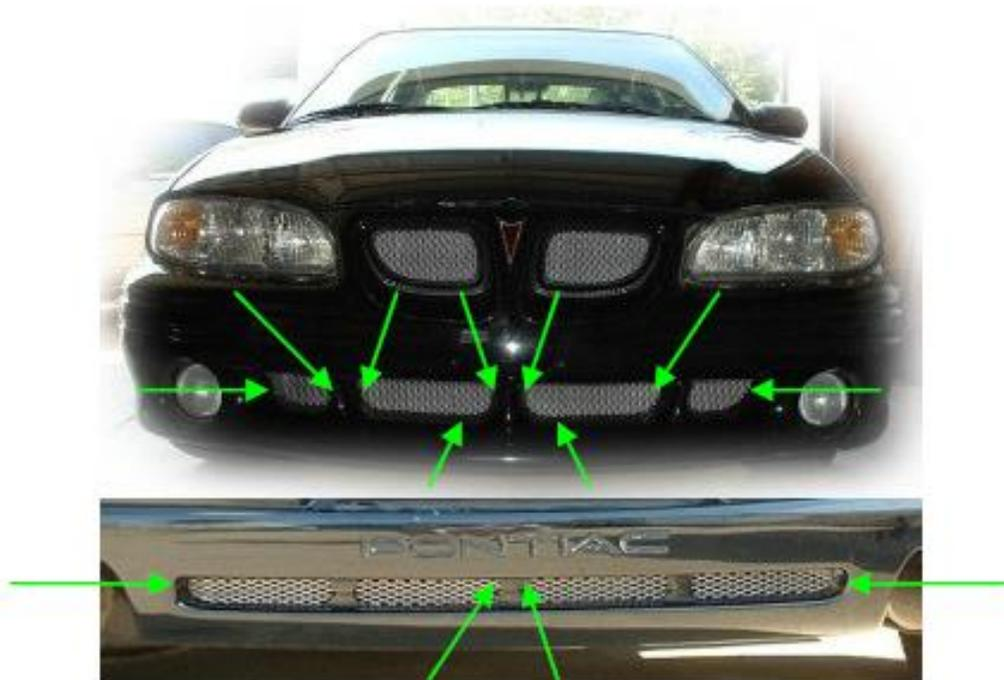
9. Next feed the cable ties through the holes using the tail end first.
