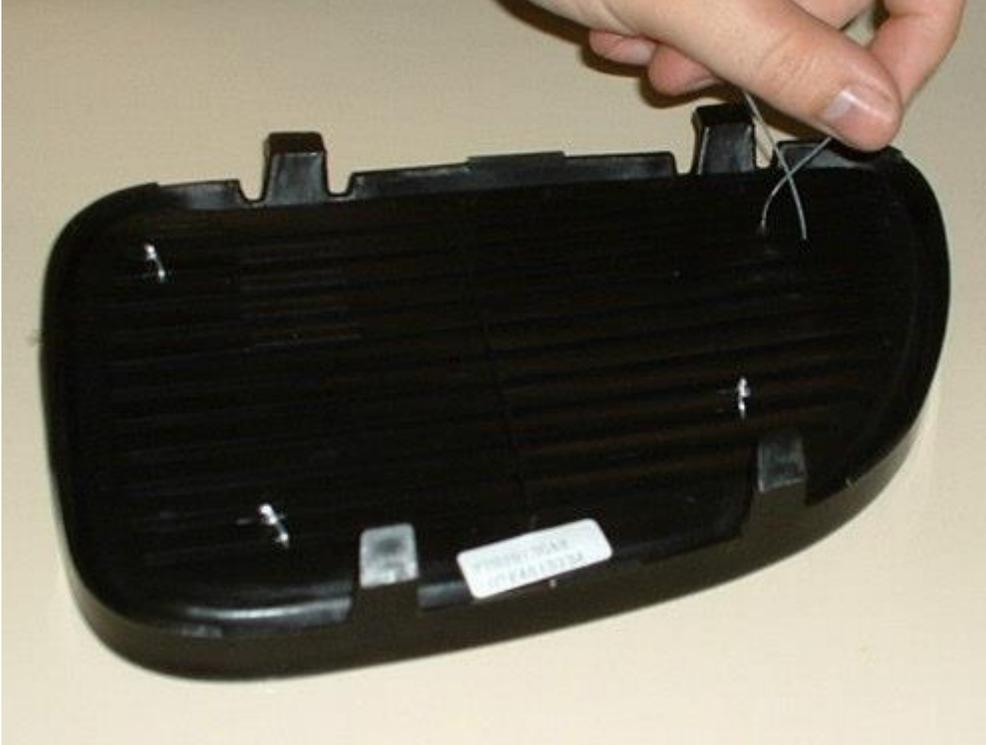
5. When you can twist it much longer, and then use a pair of need nose pliers to make a snug fit with the desired tension.
