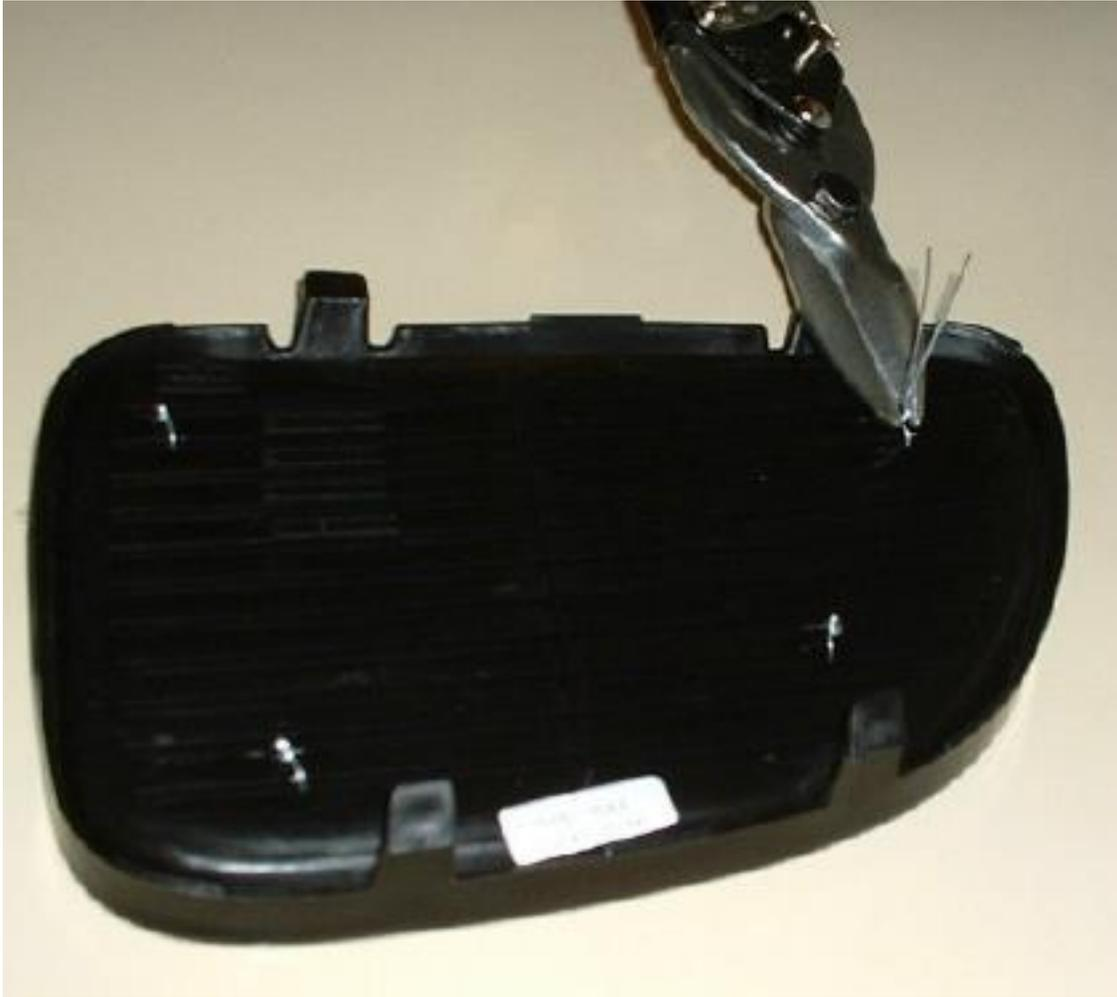
7. Reinstall the top inserts. Hook the inserts in at the top and then push the bottom tabs in to place. A common mistake on the install is having the inserts positioned too high.
