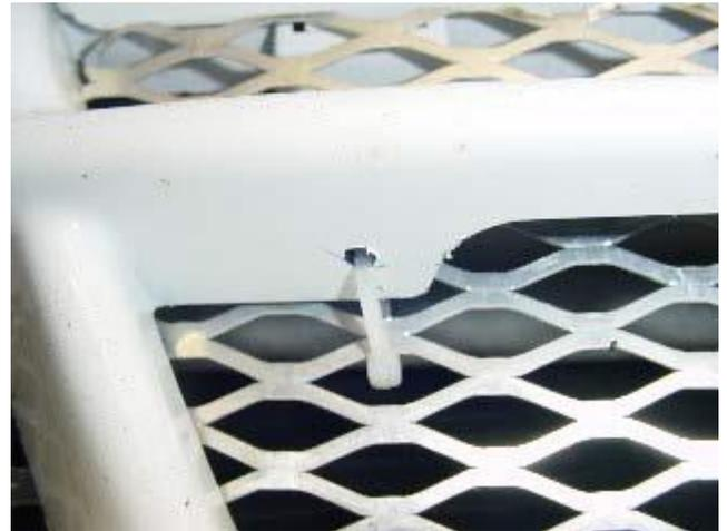
Just run the zip tie through the hole, around the mesh and tighten. Cut off the remaining length of zip tie. Do this for each hole that you drilled. If done correctly the zip ties are not visible from standing view.
