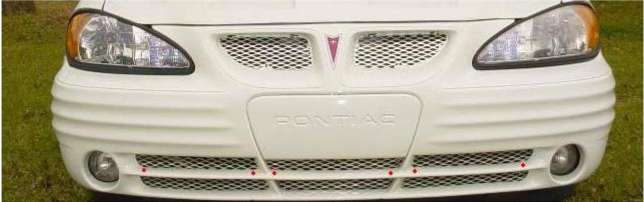
Here are some close-ups of the holes for the zip ties. The hole only has to go only through the bottom layer of the piece.
