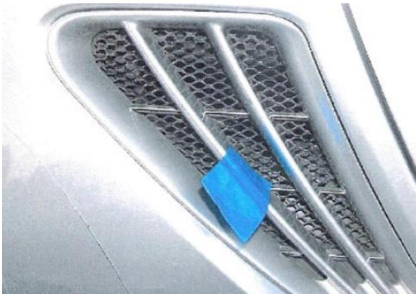
Then, insert a small flat-bladed screw driver between the ventilation grill and the retaining frame at the point indicated in the next photo (photo # 3).
