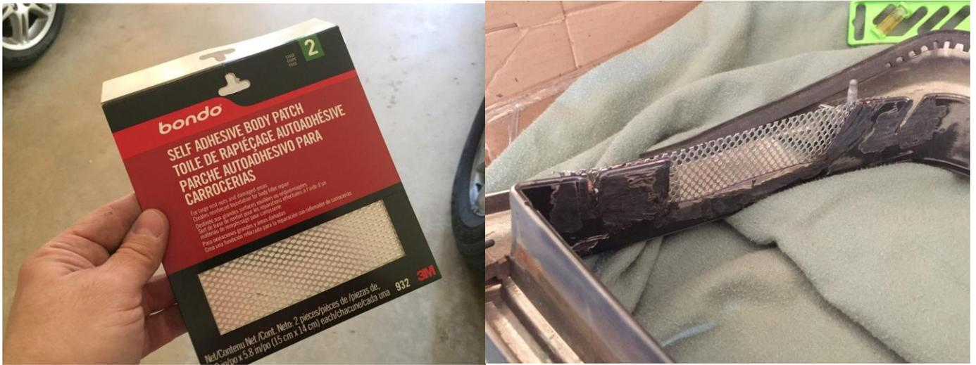
The next step is to use your choice of body filler to cover the backing material in the gaps and any other imperfections on the inside surface.
