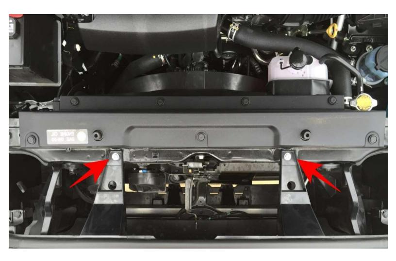
Next, use a small flathead screwdriver to pop up the pins on the retainer clips, shown below. These are just inside the light housings, behind the grill. Once pins are popped up, remove them and set aside.
