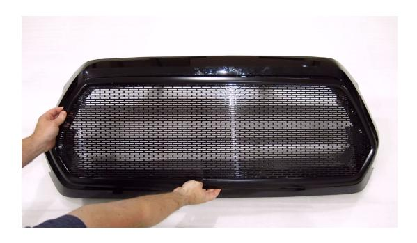
Line the tabs of the new grille up and press it in place until the tabs click.
