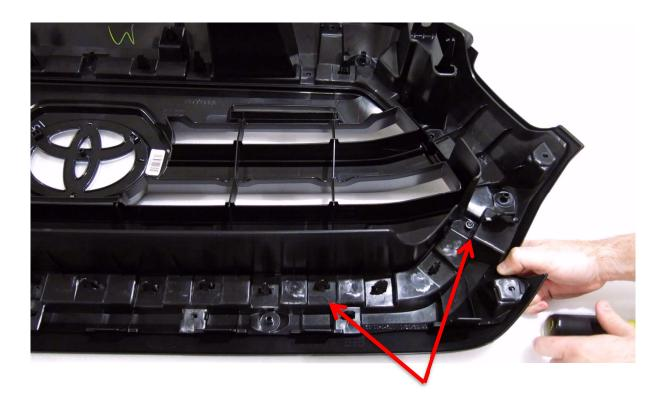
On the back of the grille, remove the small Phillips head screws that are holding the bezel in place.
