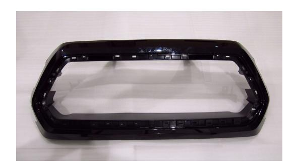
The grill shell should be hollow now and ready for the new grille to be inserted.
