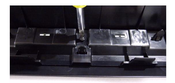
Re-install the bezel screws that were removed in an earlier step.
