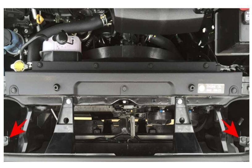
Once the fasteners are removed, set them aside. A slight tug forward (away from the truck) on the bottom and top of the central grill assembly, it will come off. Be careful not to drop it!
